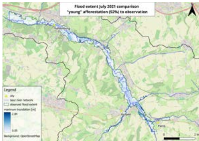
Figure 17: observed and simulated flood extent in zoomed-in area for "young" forest parameterization
