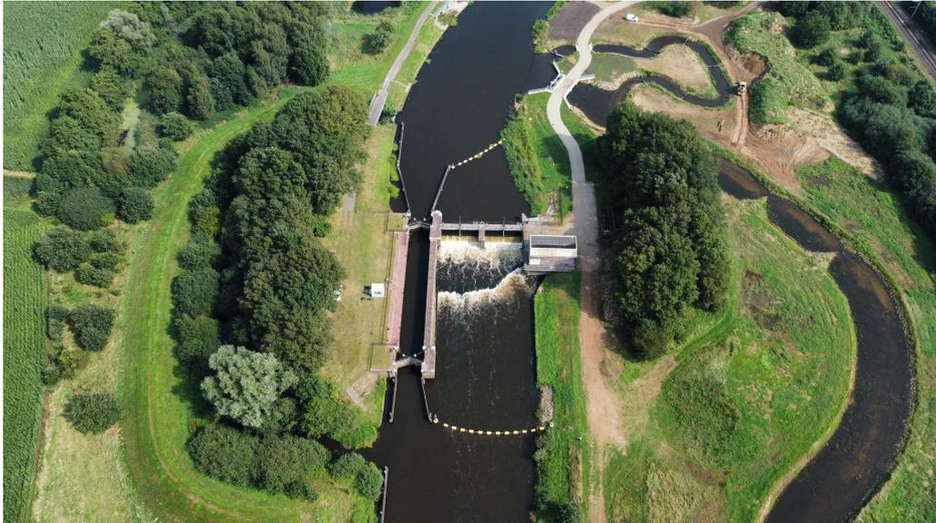
Figure 3: Weir De Haandrik in the Vecht and recently developed fish ladder (right). Photo: William Cazemier
